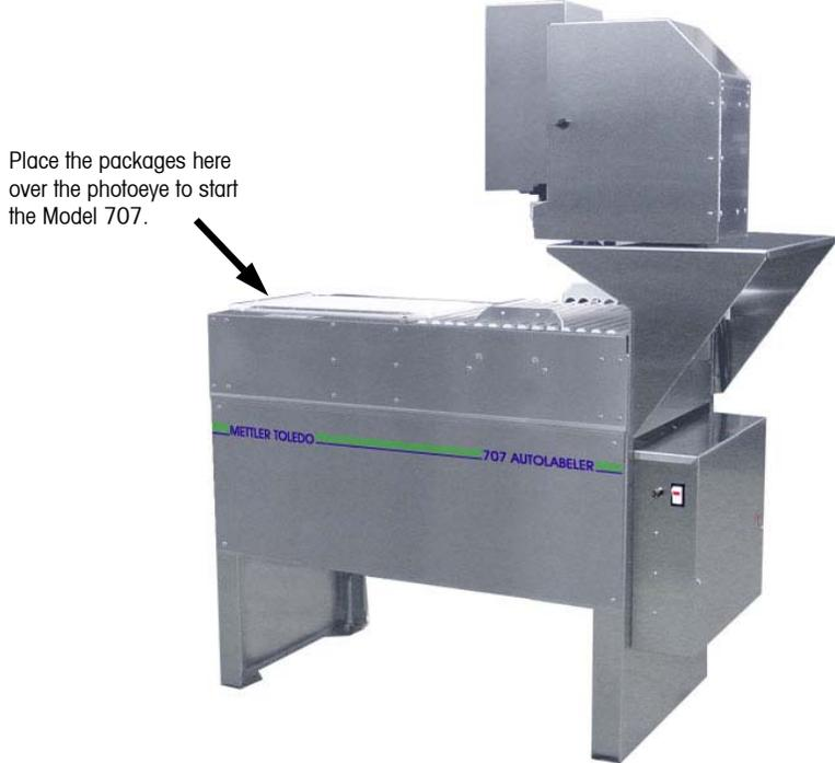
Figure 2-1: Manual Feed (without Indexer)
